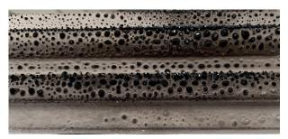
Coating after approx. 5 min. of fire load.
