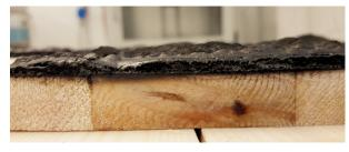
The fire-retardant coating (DIN EN 13501-1) foams up and forms a temporary barrier to the flames.
